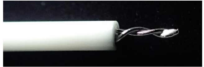
Fig.2: A twisted tip of the FlexIr-TC.
